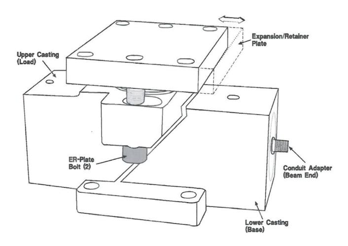
Figure 2-1. The Z-BLOK Weigh Module
