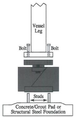
Figure 2-3. Z-BLOK Installation Assembly Diagram
